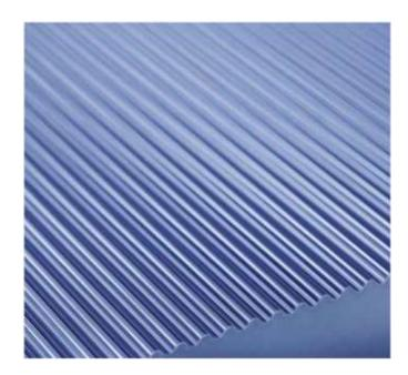
The LSP consists of linear prisms which are modified sinusoidally in their cross section so as to function as an optical diffuser perpendicular to the main axis of the sheet. The main ray path is maintained in order to ensure high efficiency in comparison with standard opal materials.
