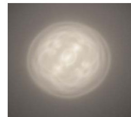
Spot From Collimated Light (no diffuser)
