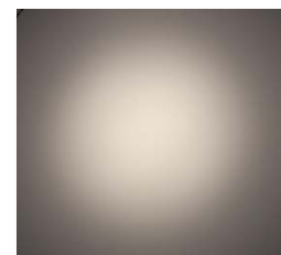
Collimated Light with M-Series Mixing Diffuser
